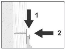
First place the clip over the plank; then screw/rivet into place.
