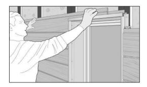
Allow minimum 10 mm gap at window/door head and sill interface for ventilation.
