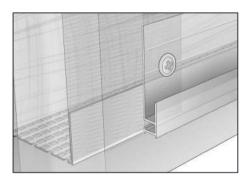
The starter profile is installed over the ventilated profile.
