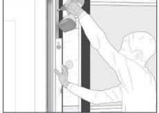
Depending on the project detailing and requirements, external corner profile may be used as a jamb profile at openings (doors/windows). In this or similar case, where the profile meets a lintel profile above the opening it may be notched accordingly for a neat finish.
