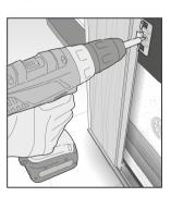
First Cedral Click plank is installed truly straight with the tongue side facing where the next plank will be located.
