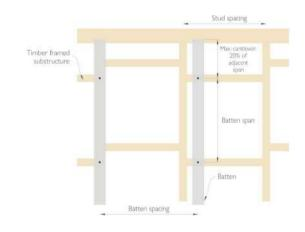
Table 4 – Timber batten span with respect to wind category – Cedral Click Horizontal For buildings within the scope of NZS 3604
