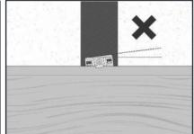
Screw (or rivet in case of fixing to metal) the clip into place using the matching screw/rivet (supplied with the clips) to ensure that it remains pressed tightly to the strip and is level with it. Slightly incline the screw if necessary, so it pushes the clip down when fixed.
