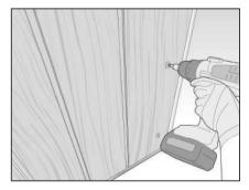
The first and last planks are face fixed using Cedral face fixings on the clipless side of the plank with adequate edge distance.
