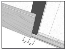
Make sure that the plank end aligns with the middle of the vertical batten (support frame).
