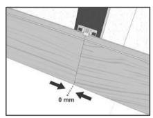
Mount the next plank. Place abutting planks in such a way that the ends touch (no gap) and they always meet on a support frame profile. Planks should be loosely butted (no force).
