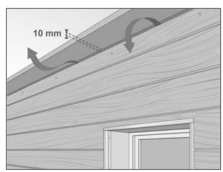
Min. 10 mm gap is required at the top of the façade for ventilation.
