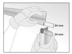
Notch the corner profile where meeting a lintel profile. The lintel profile may need to be cut longer on the flange located on the opening reveal; refer to Cedral Construction Details fro further details.
