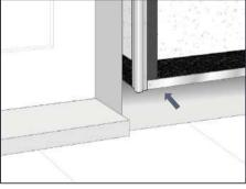
Ensure the bottom of the external and internal corner and end profiles are flash with the installed ventilated profile which indicates bottom of the cladding.
