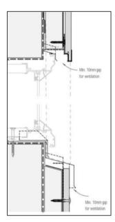
Ensure ventilation gaps are allowed at window/door heads and the like. For full details refer to Cedral Construction Details documents.
