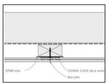
The clip must be centred at the butt joint
