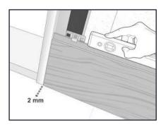
Position the first plank on the starter profile, keeping a 2 mm gap. Fit the bottom of the strip into the profile. Slide the Cedral click clip onto the strip. Provide one clip at every batten.
