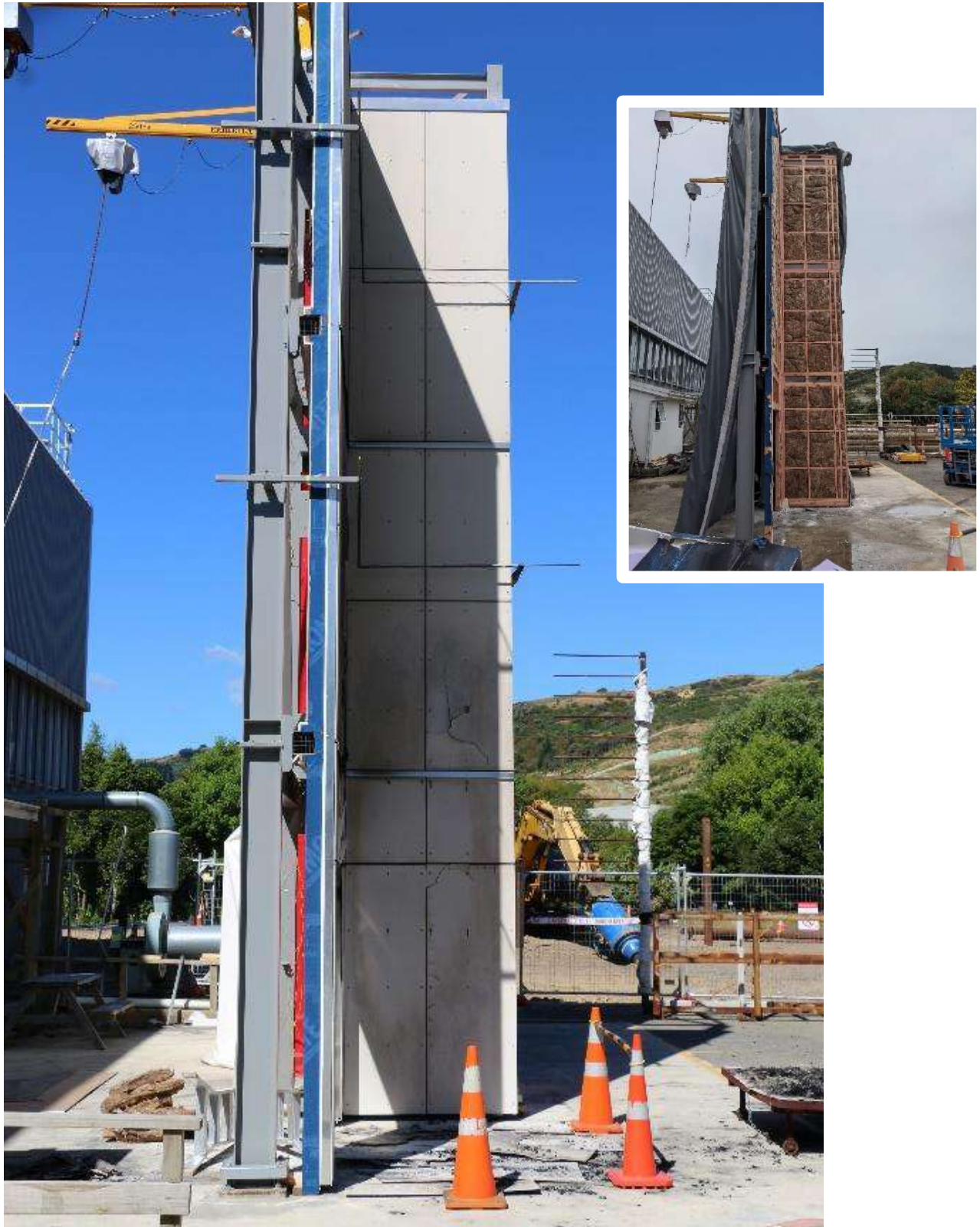
Photo 33: Post-test wing wall cladding, inset: timber frame
