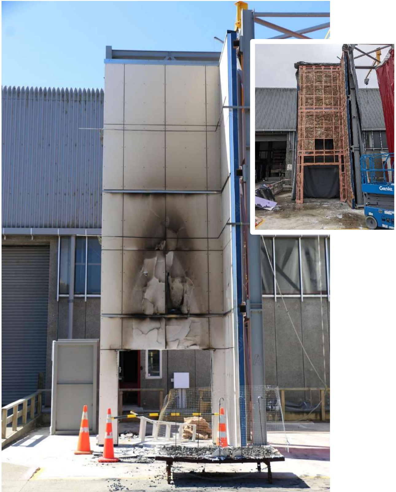
Photo 32: Post-test main wall: cladding, inset: timber frame
