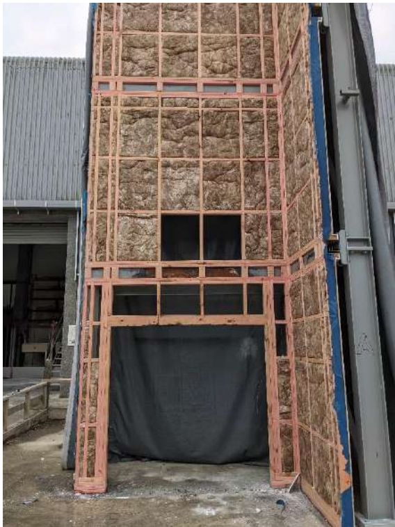
Photo 2: Timber frame and insulation (Missing sections of insulation removed by BRANZ post-test).
