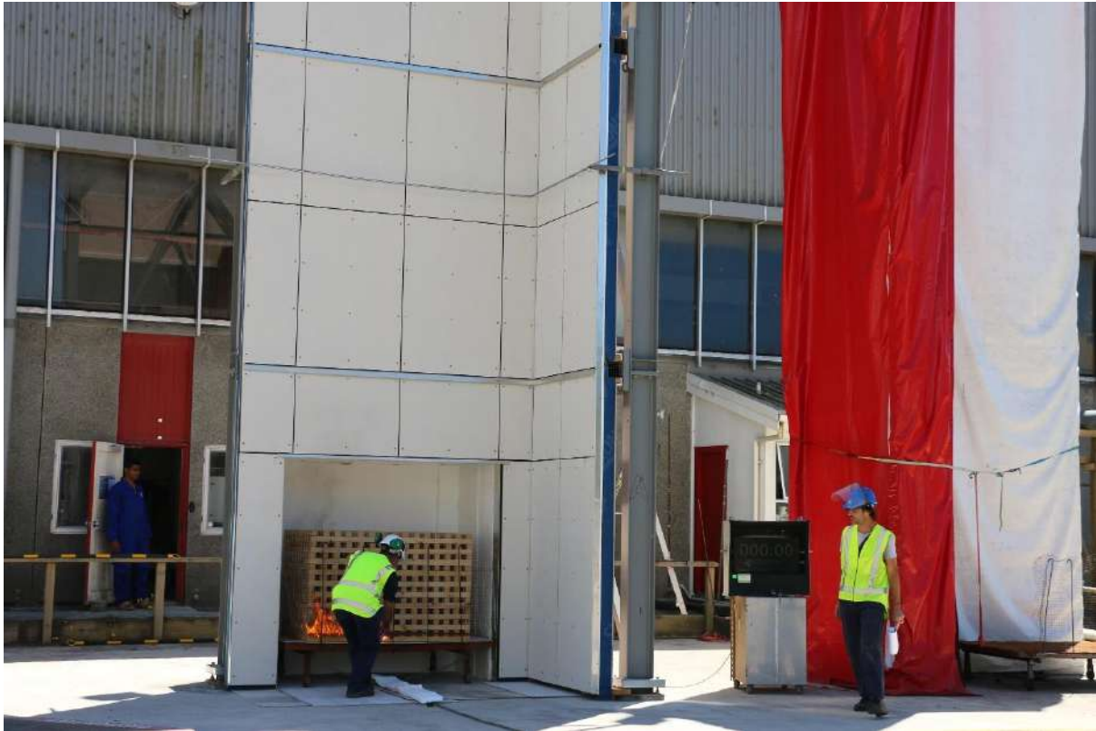
Photo 20: Ignition of timber crib
