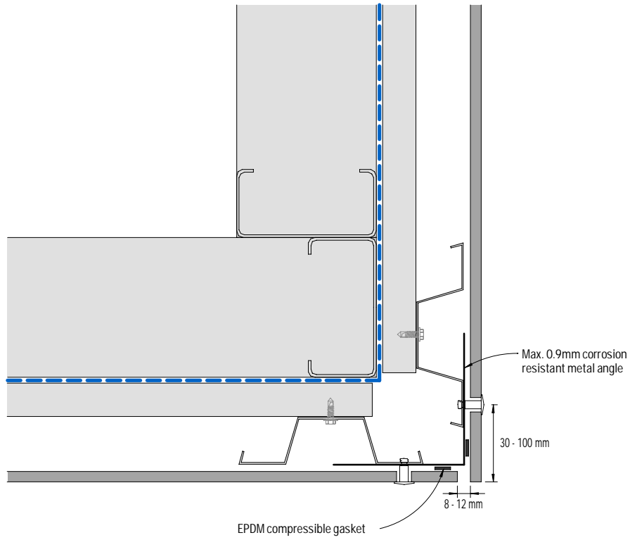
Figure 27: External corner - Detail 1
